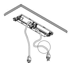
Note: In a conduit application, conduit should be supported according to local code. When managing conduit and cabling exiting the unit, ensure there is adequate slack to allow unit to open properly.
