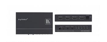
The VM-22H is a distribution amplifier for HDMI signals. The unit reclocks and equalizes one of two selectable input signals and distributes it to two identical outputs.
