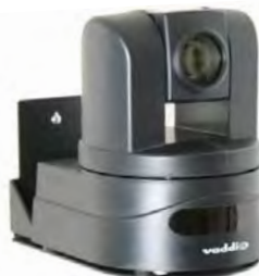
Fig. 8: Vaddio HD-18 Camera aligned and attached to the CONCEAL Wall Mount Bracket (by two-(1/4"-20) screws in the bottom of the mount)
